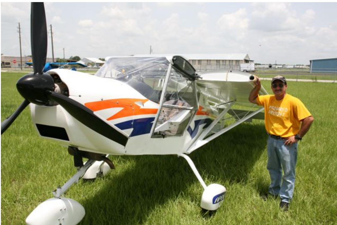
Wings folded by one person in less than 10 minutes
